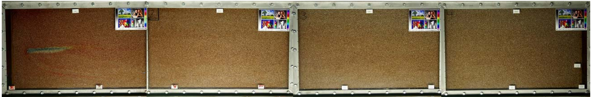
Figure 5. 11 Reactive-mixing plume with a 2.10 cm injection source width (experimental data)
