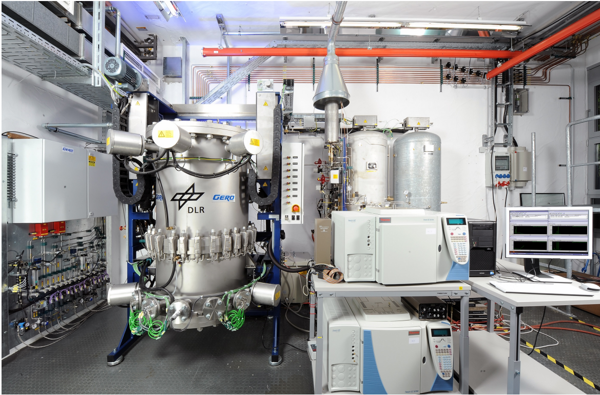
Figure 3.1: Laboratory with pressurised SOFC test rig including gas distribution (left), pressure vessel (centre), equalising tanks (back), and gas chromatographs (front right) [90].
