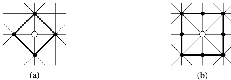
Figure 5.4 The surrounding polygon ( thick line ) of a vertex ( \circ ) with (a) four neighbors and (b) eight neighbors.
