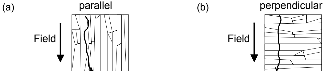
Figure 6.15: Conduction parallel (part (a)) to grains, and perpendicular to them (part (b)). The electrons paths sketched with the thick, curved lines, show that when the transport is perpendicular to the grains, the electrons will encounter more grain boundaries, resulting a higher resistivity.
