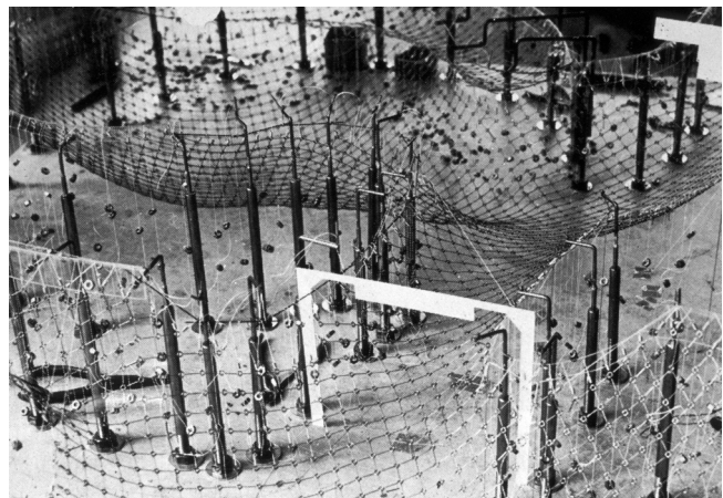
Detail of the form-finding model [IL 13]
