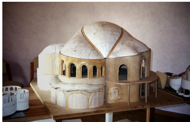
Designing model for the "Hölderlin-Haus", Maulbronn, made of wood and gypsum in scale 1/20
