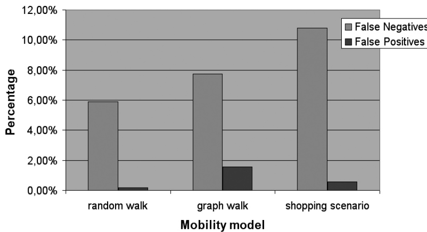
Figure 7.32: Percentage of false positives and false negatives for mobility traces generated from different mobility models
