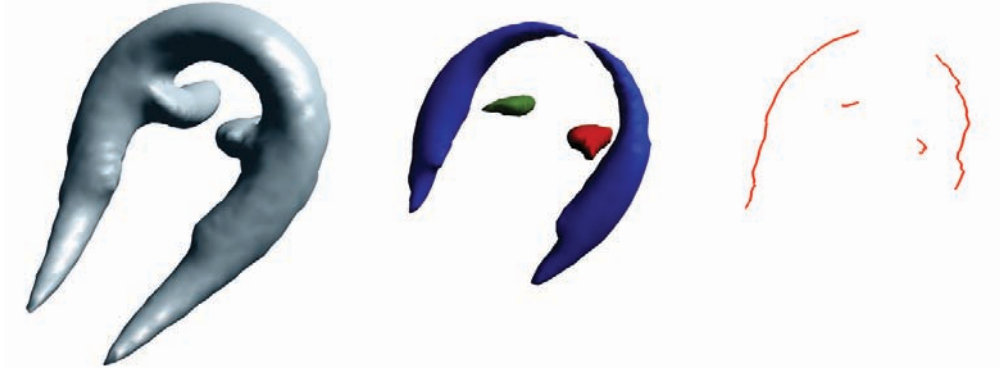
Figure 8.9: Semi-automatic isovalue determination: original vortical region (left); decomposition with color coding by isovalue (middle) and \epsilon = 5\% ; the respective vortex core lines (right).
