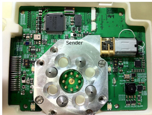
Figure 2.12: The active docking element of the robot from Karlsruhe.
