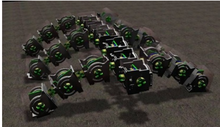
Figure 2.4: A picture of a multi-robot organism. The 24 single robots are connected to one big organism called hexapod. [Sym10]
