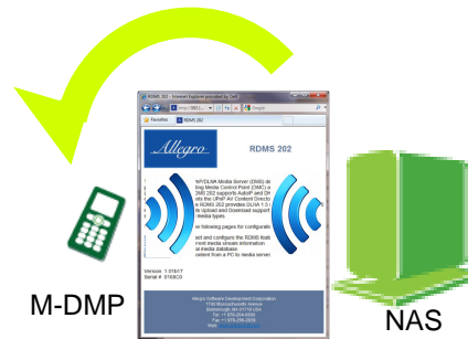
Figure 4.21.: Touch the phone with a NAS, users will get the presentation page of NAS on the phone
