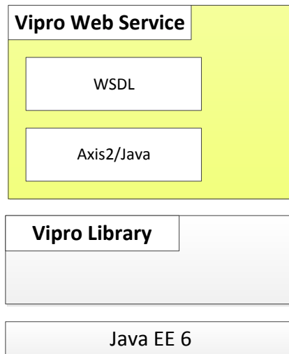
Figure 29. Components diagram for Vipro Web service.
