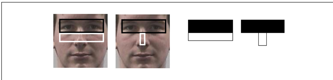
Figure 2.13: Typical Haar-like features for frontal face: The typical features for frontal face expect that the eyes region is darker than the nose bridge or the upper part of the cheeks.
