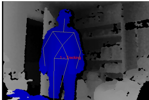
Figure 2.3: The Kinect detects any person and tracks it. The position of several joints form every active player are calculated resulting in a skeleton.
