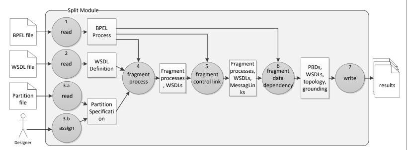
Figure 7.3: The full splitting module
