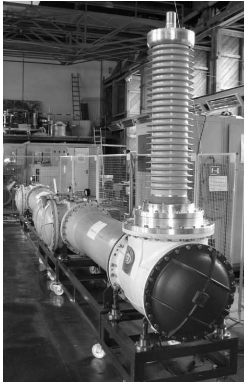
Figure 8: The high voltage test setup in the laboratory of University of Stuttgart: ABB 550 kV GIS type ELK-3 with bushing
