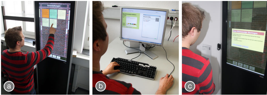
Figure 9.12: Study Arrangement: (a) Digifieds display client, (b) Digifieds web client on PC, (c) Scanning QR code from paper.
