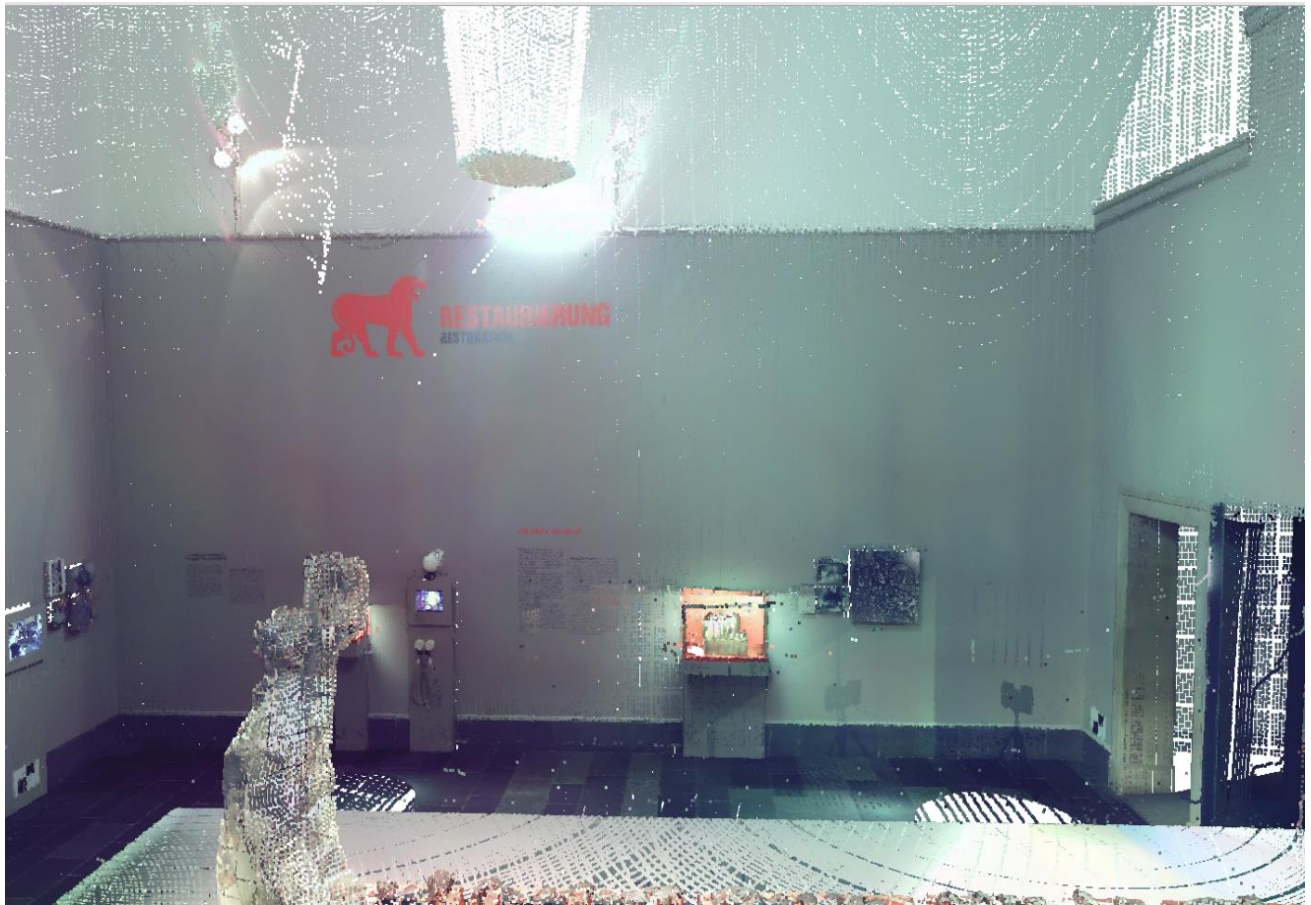
Figure 5.13 Final Point Cloud after Color Transfer with Interpolation
