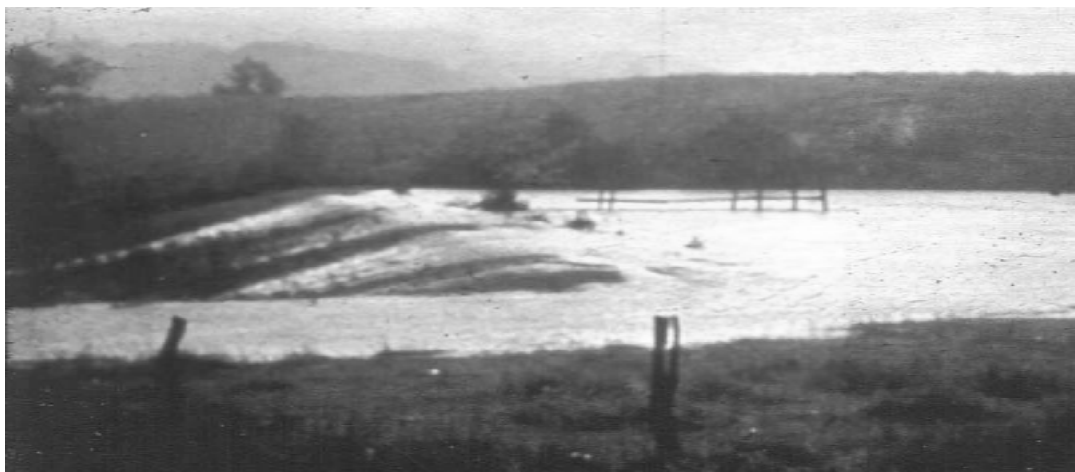
Figure 2.7: Overtopping failure of an embankment dam [36]
