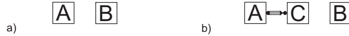
Figure 3.3: a) A declarative workflow is implicitly modeling arbitrary execution orders of two tasks. b) The restructured workflow after adding a new task (C) that has to be executed directly after task A.
