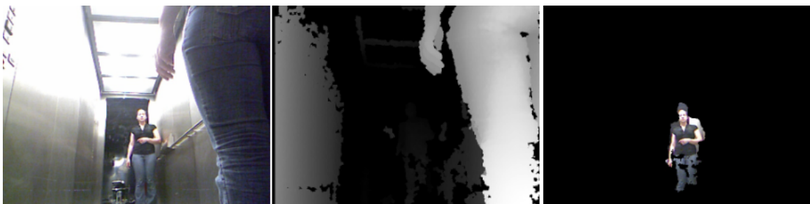
Figure 4.7: Mirror taking effect on guide recognition and “hijacking” the robot.
