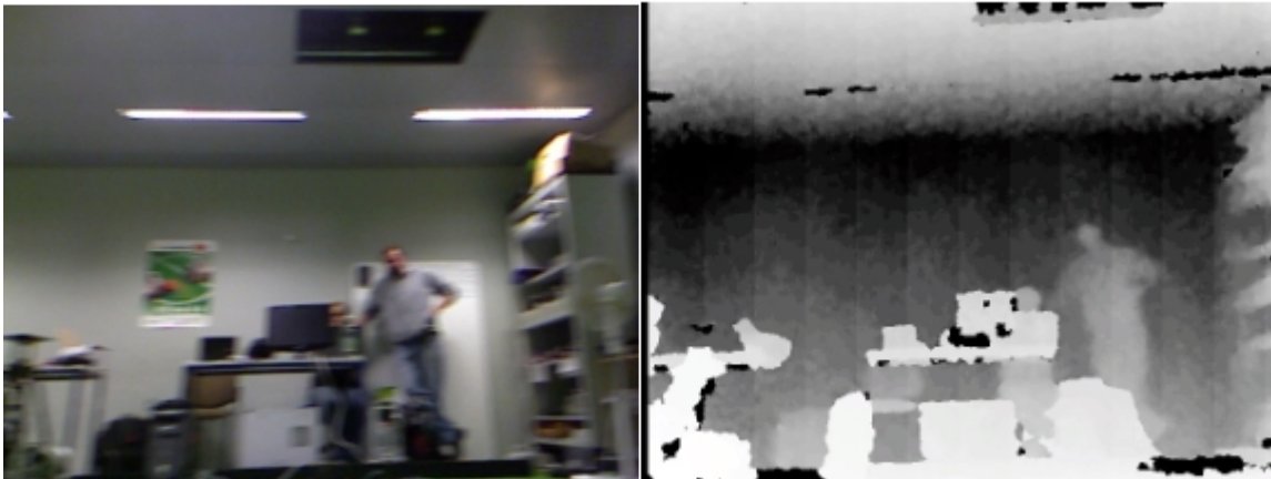
Figure 4.3: Images are result of rotation of the robot with Microsoft Kinect. Even this minor motion blurring suffices to loss guide recognition
