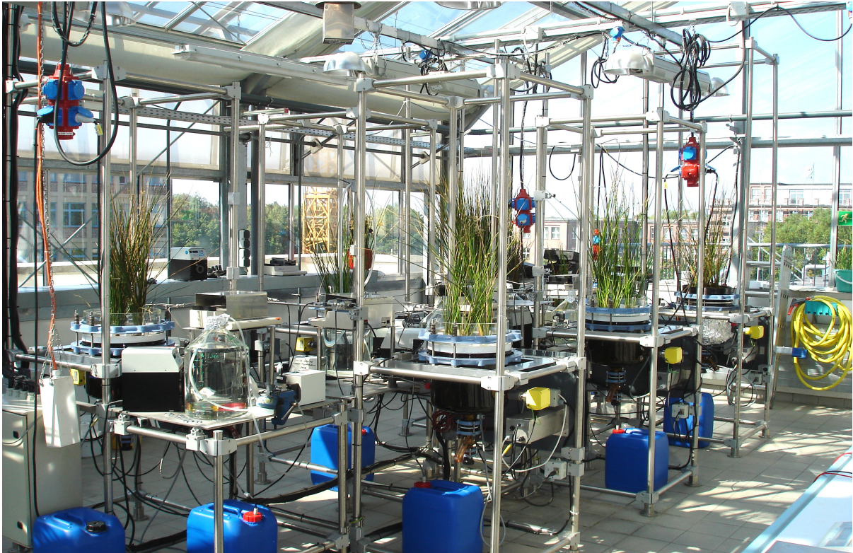
Figure 3.2 Experimental set up of the Planted Fixed Bed Reactor – PFBR
