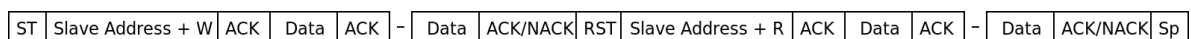
Figure 2.8: Sequence of combined transmission with the help of the repeated start signal
