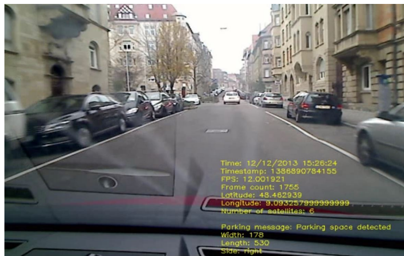
Figure 7.3: The Java program grabs each frame from the webcam and each time a parking space is detected, GPS location is read and textual information is added to the frame; also the parking space data is saved in a separate log file
