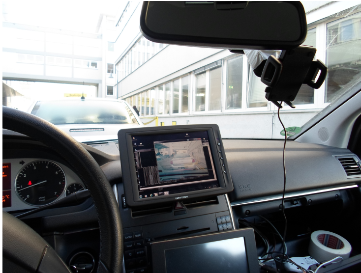
Figure 7.2: The webcam that records the frontview is mounted on the windshield of the vehicle and the code that logs and records the video is running on the car PC
