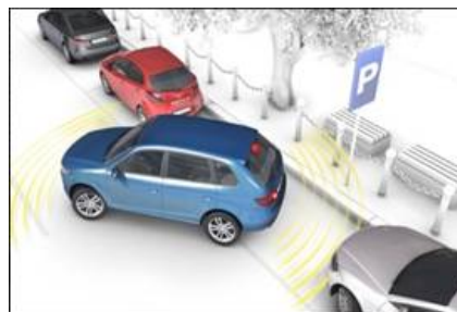
Figure 3.3: Vehicle doing reverse parallel parking maneuver with the support of semi-automatic parallel parking using ultrasonic sensors (Source: Bosch GmbH)
