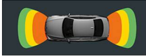
Figure 3.2: Visual output of ultrasonic sensors shows different colours around the car according to how close the surrounding objects are located from the vehicle (Source: Bosch GmbH)
