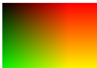
Figure 5.1.: A sample correspondence map showing the mapping of each pixel to itself. The R component contains the x coordinate, G the y coordinate. B is always set to the value of 1.0 for consistency reasons.
