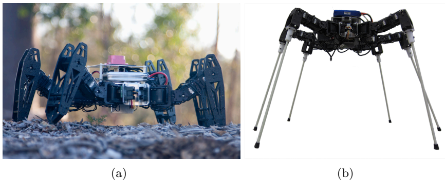
Figure 9.1: Modified PhantomX hexapods (a) with additional computing and sensing, (b) with extended tibia segments for reduced stability.
