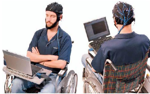
Figure 3.6: Mind-controlled wheelchair using a brain-computer interface for drive command classification [Bal09].
