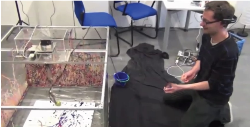
Figure 3.7: Painting robot called roboPix. roboPix draws action paintings based on thoughts and the emotional state of a user [FR13].
