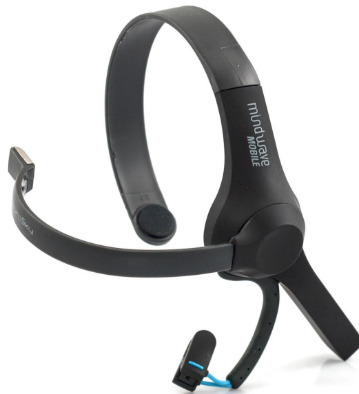
Figure 4.7: The wireless, non-invasive and single passive dry sensor EEG, NeuroSky Mind-Wave Mobile a .
