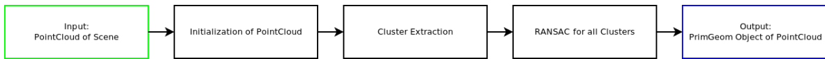
Figure 4.1: Overview of second approach of representing a point cloud as a PrimGeom object.
