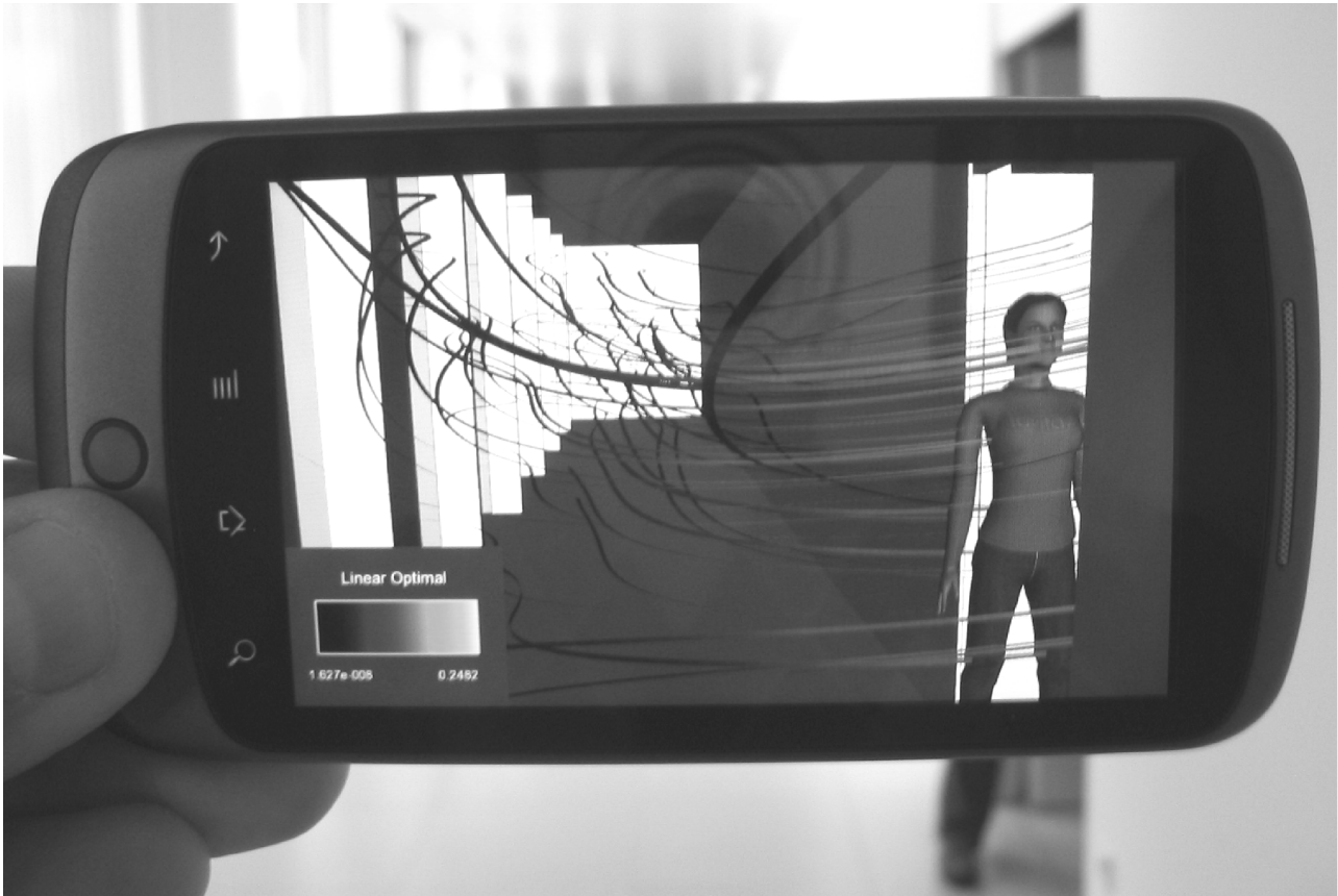
Figure 2.1: Real-time Flow Visualization of Stream Ribbons which shows the airflow in a building based on the user's current position. [42]
