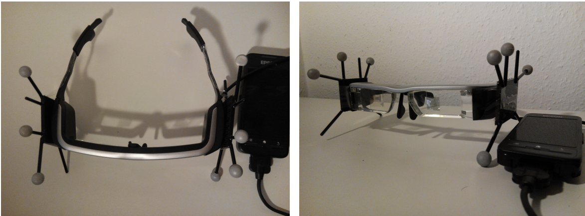
Figure 4.2: The Epson Moverio BT-200, equipped with passive infrared tracker for the motion tracking system.
