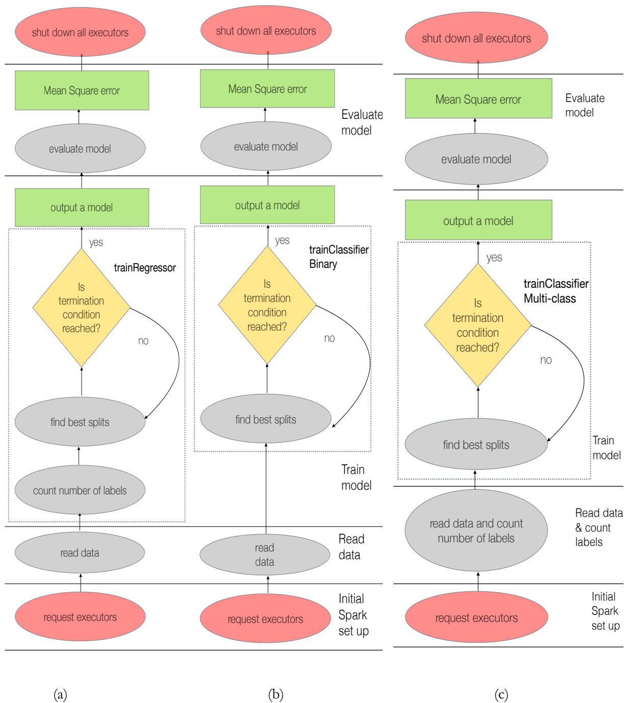
Figure 23. Stages in decision tree learning for regression and binary classification in MLlib
