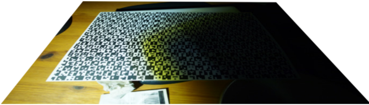
(a) Input image with strong perspective distortion, note low resolution and the difficulty to make out the bit patterns for markers at the far end.
