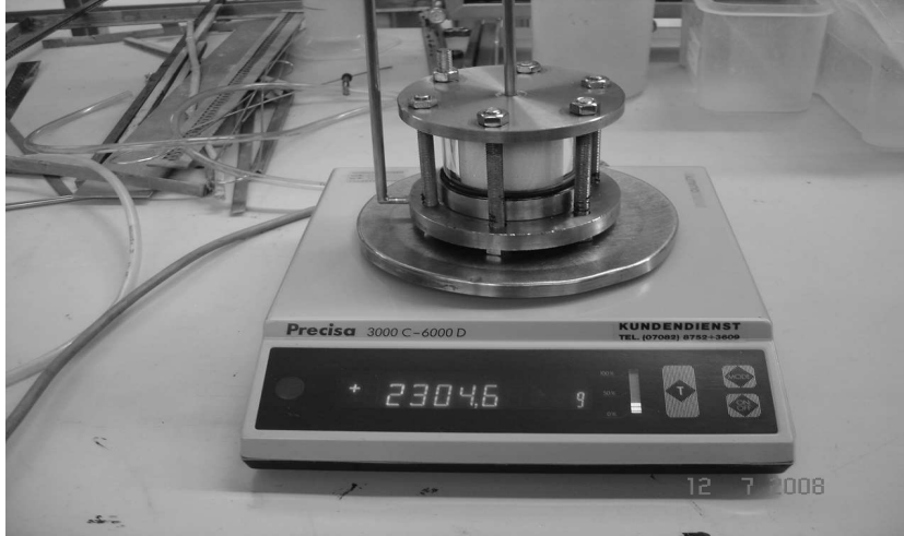
Figure 4.3 Device used to measure h_c - S relationships of fine and coarse glass beads.
