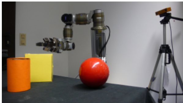
Figure 5.7: Experimental setup: Schunk 7-DoF arm, Schunk 7-DoF hand, Bumblebee stereo camera, coloured objects with various shapes.
