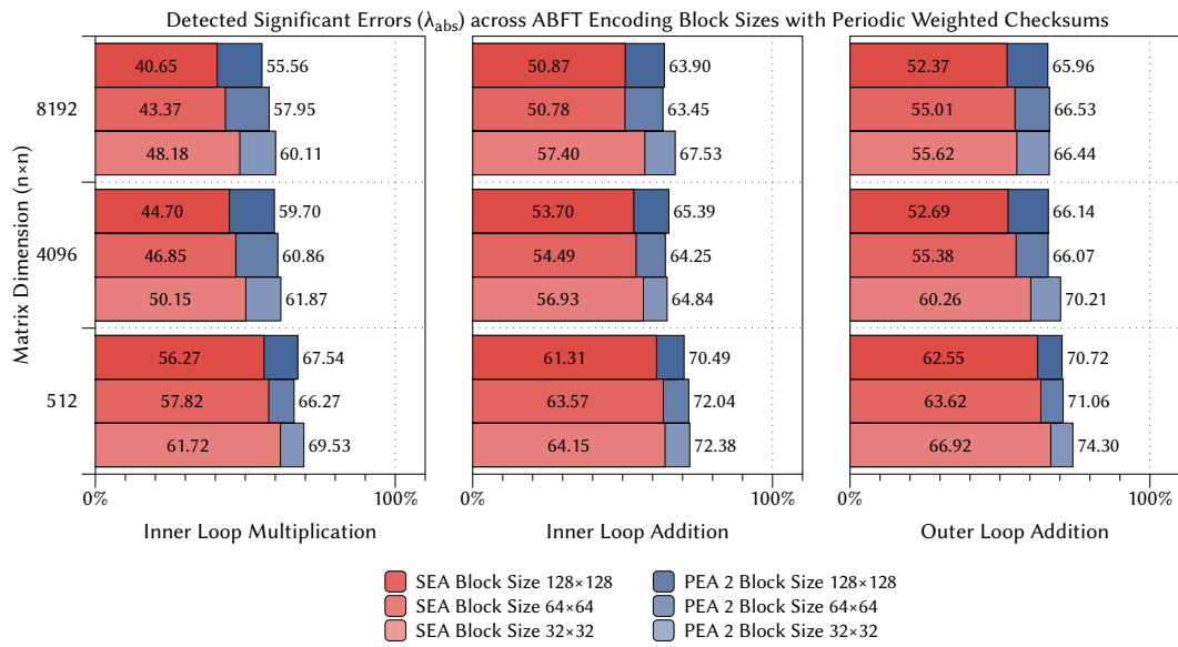
▲ Figure F.13 — Detected significant errors ( \lambda_{abs} ) across different ABFT encoding block sizes for periodic weighted checksums and test data set T_{ortho}(0,65536) .
