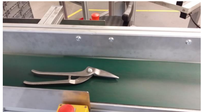
Figure 23. Example of how the shears should be placed on the belt.
