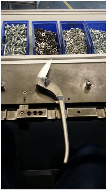
Figure 17. Example of how the screw should be linked through the bottom half of the shears.
