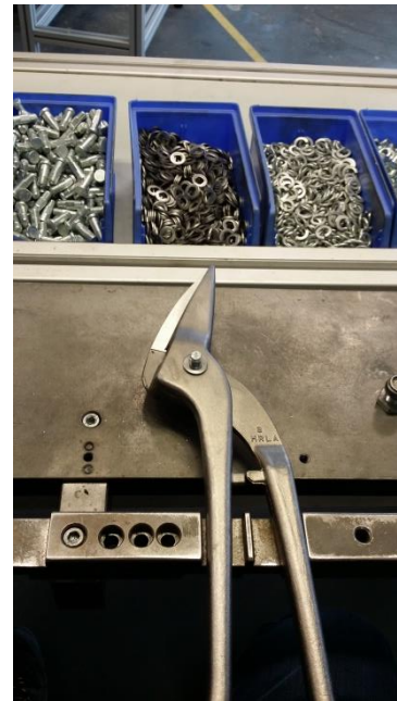
Figure 19. Example of how the washer should properly sit on the shear-halves.
