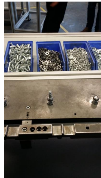
Figure 16. Example of how the screw should be attached to the production platform.
