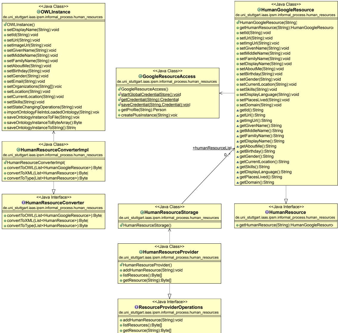
Figure 6.2: HRP architecture as an UML class-diagram.
