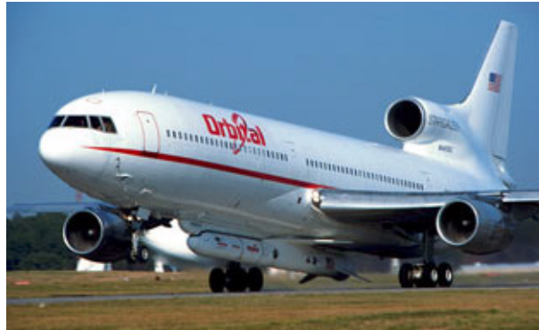
Fig. 2.1: Launch of a Pegasus vehicle carried by a L-1011 airplane Photography by courtesy of Orbital Science Corp. [87]
