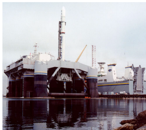
Fig. 2.2: Launch platform and command vessel. Photography by courtesy of Sea Launch Ltd. [88]
