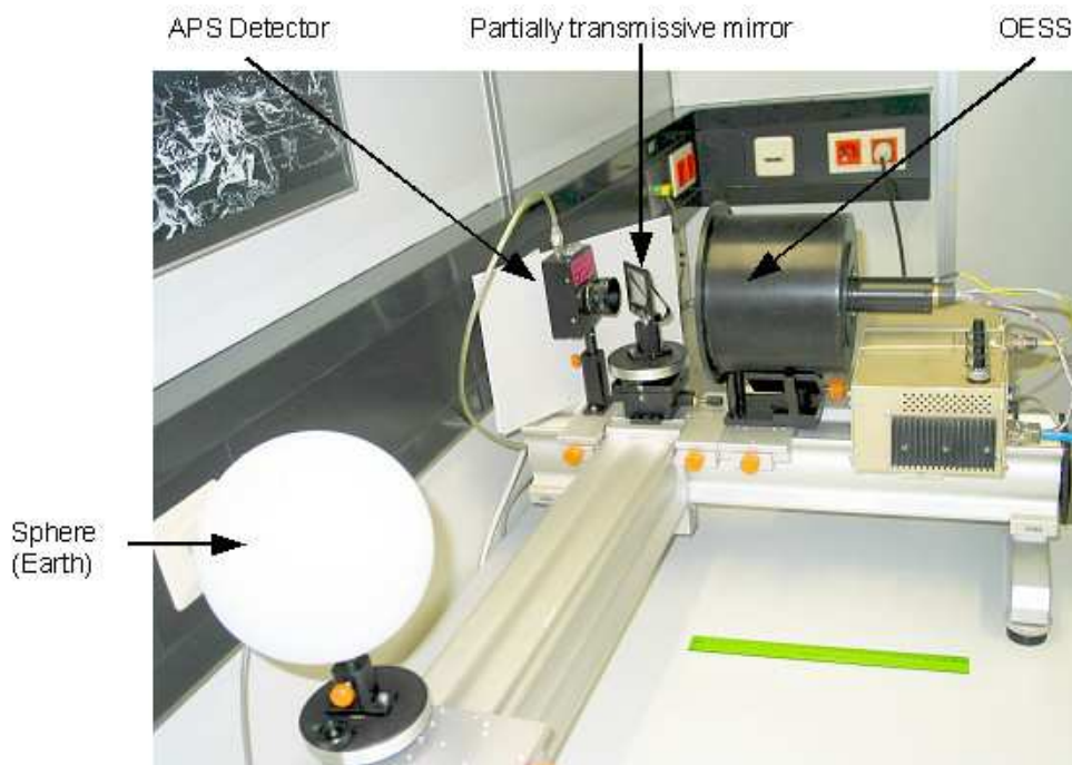
Figure 7.2: Laboratory setup as assembled and used for functional tests
