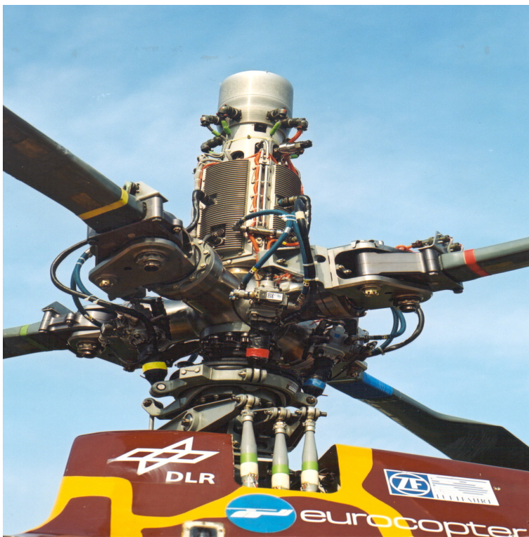
Figure 1.5 Rotor hub of BO 105 with individual blade root control system [88]
