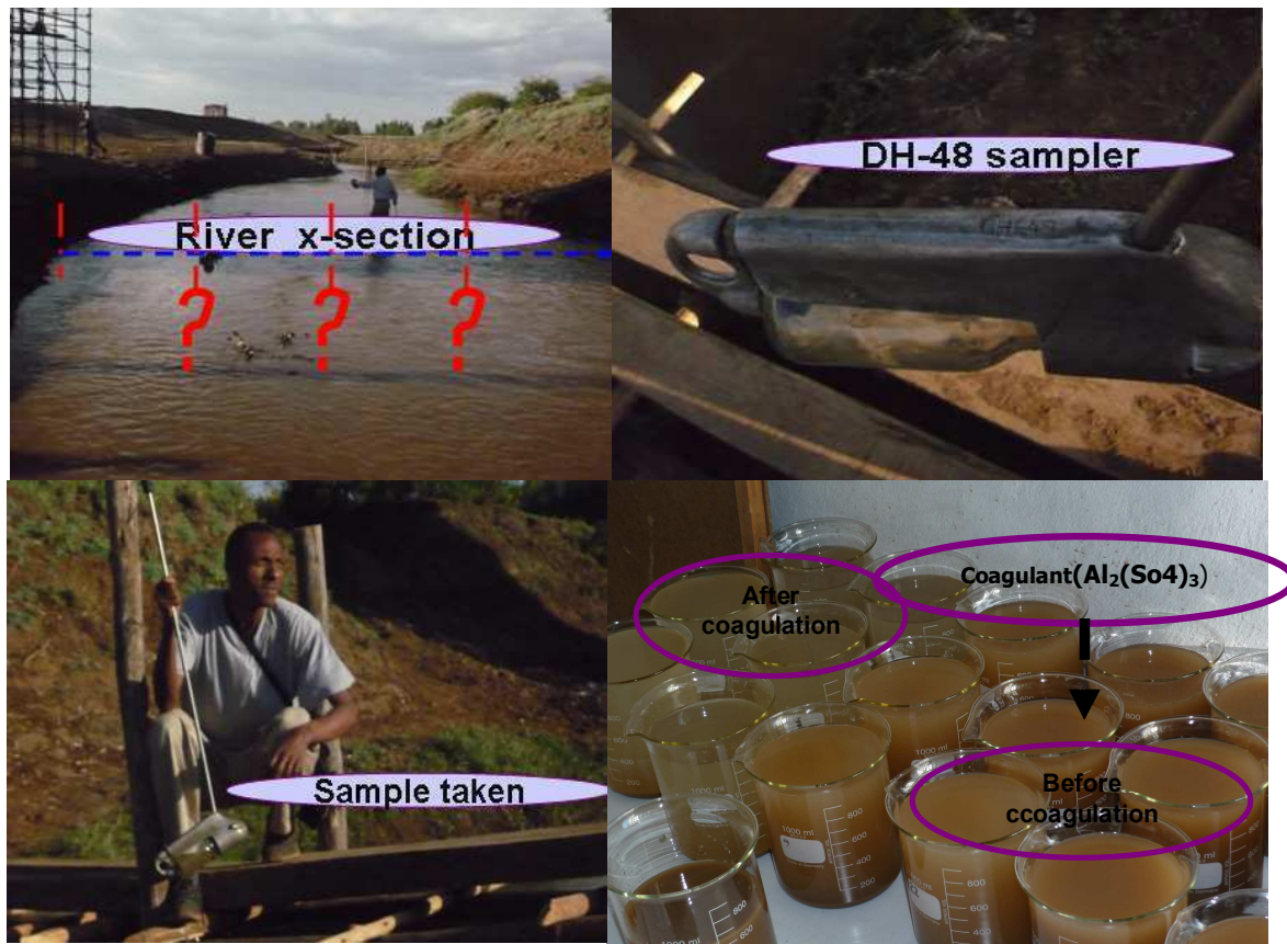
Figure 3.3: Collection and analysis procedures of suspended sediment data
