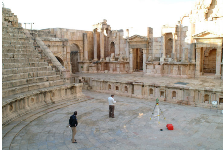
Figure 2. Data collection for the North Theatre in Jerash. The recording with the laser scanner is carried out together with surveying work using a total station.
