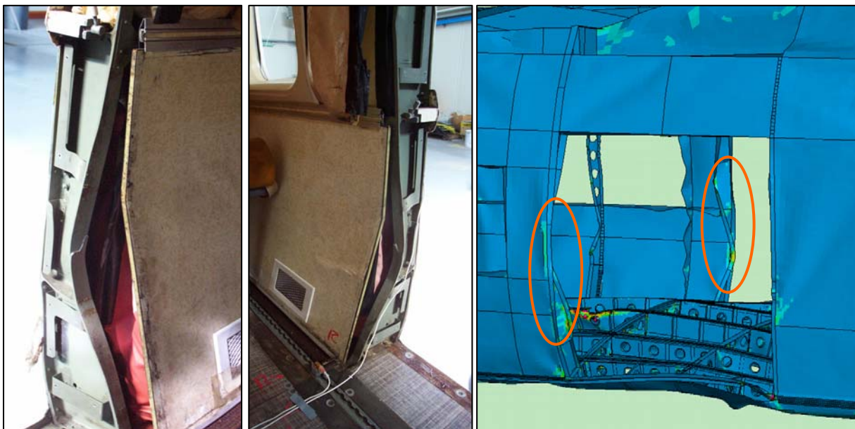
Figure 5-21 : Deformation of frame 450 on the side of each door in the simulation and after the test
