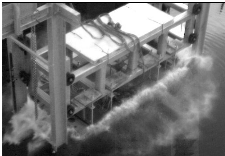
Figure 5-3 : Drop test of the WG30 sub-floor at CIRA [101]
