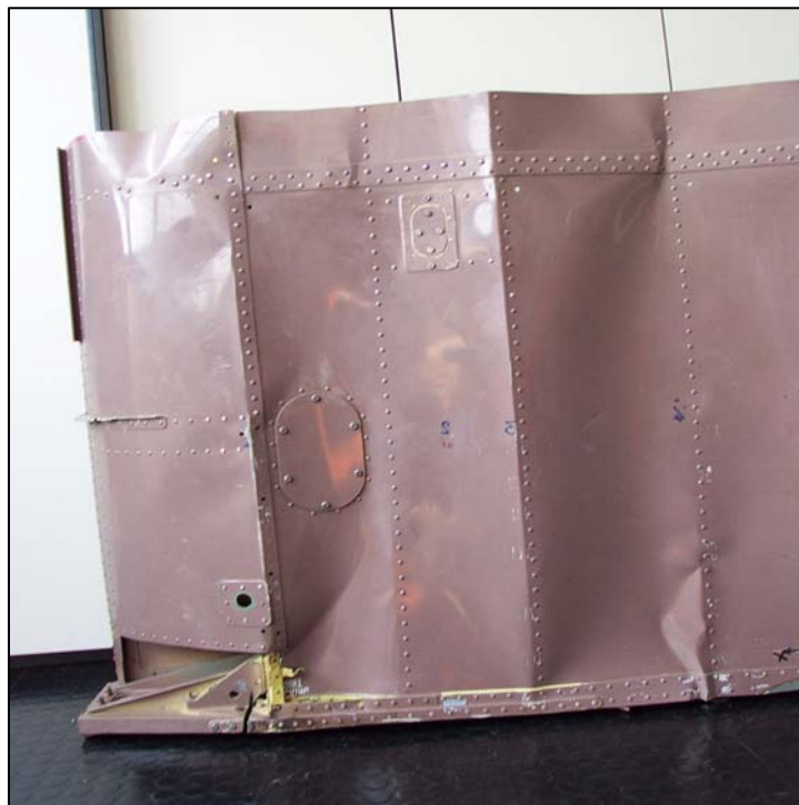
Figure D-4: Lower view of the sub-floor deformations in the analysis at t = 40 ms and after the test
