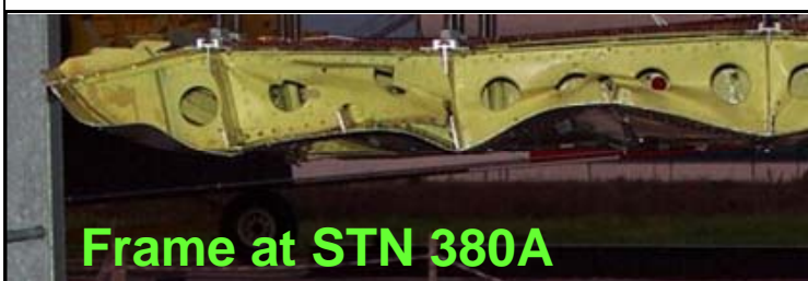
Figure D-3: Upper view of the sub-floor deformations in the analysis at t = 40 ms and pictures of the damage after the test
