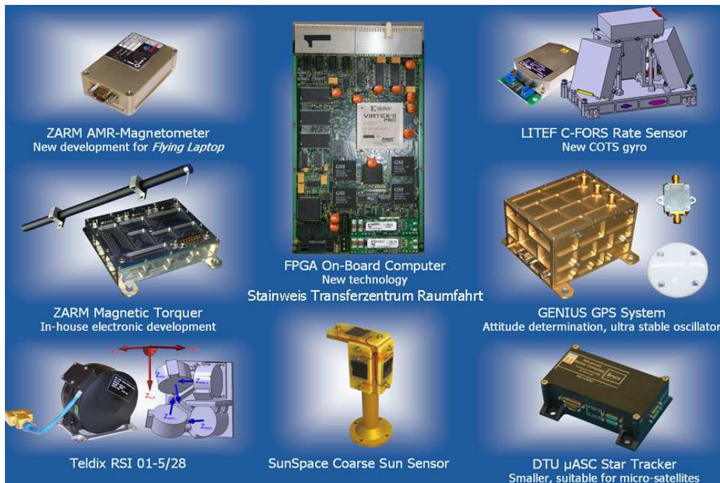
Figure 3.4.: Attitude control system hardware components
