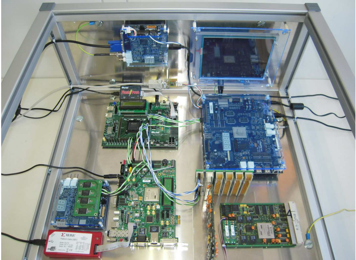
Figure 5.16.: Breadboard model of the on-board computer
