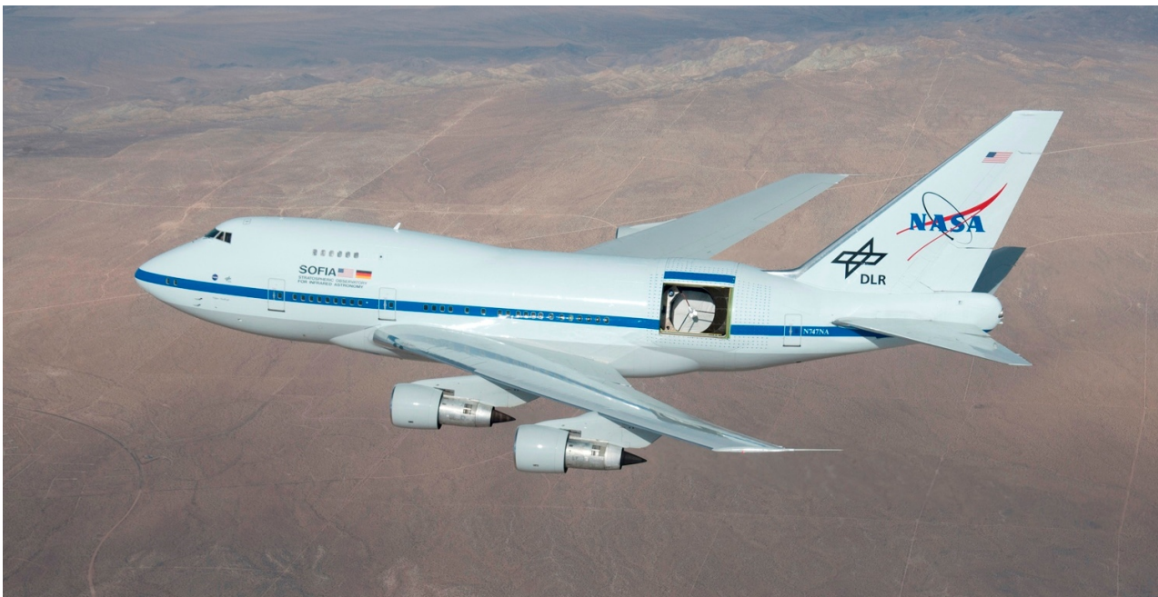
Figure 1.1.: SOFIA during its first test flight with fully opened door, December 2009.
