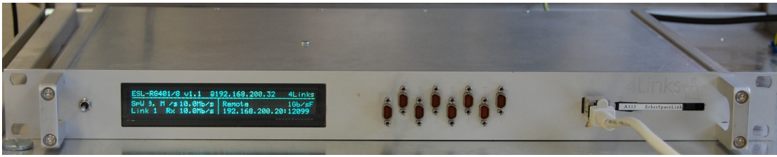
Abbildung 4.5: Ethernet SpaceWire Router
