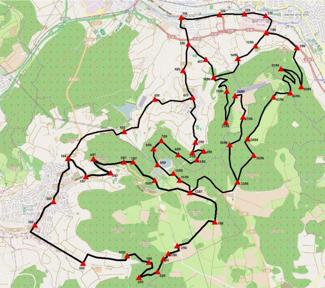
Figure 3.8 Close loops that generated from surveying paths
