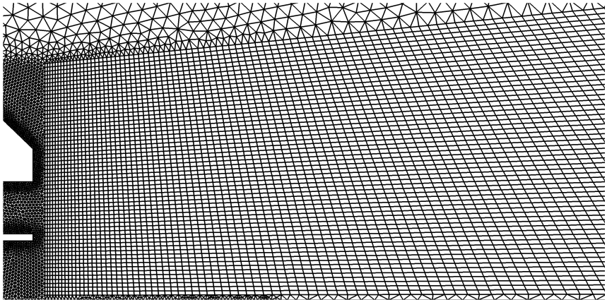
(b) Close up of structured and unstructured grid at injector.
