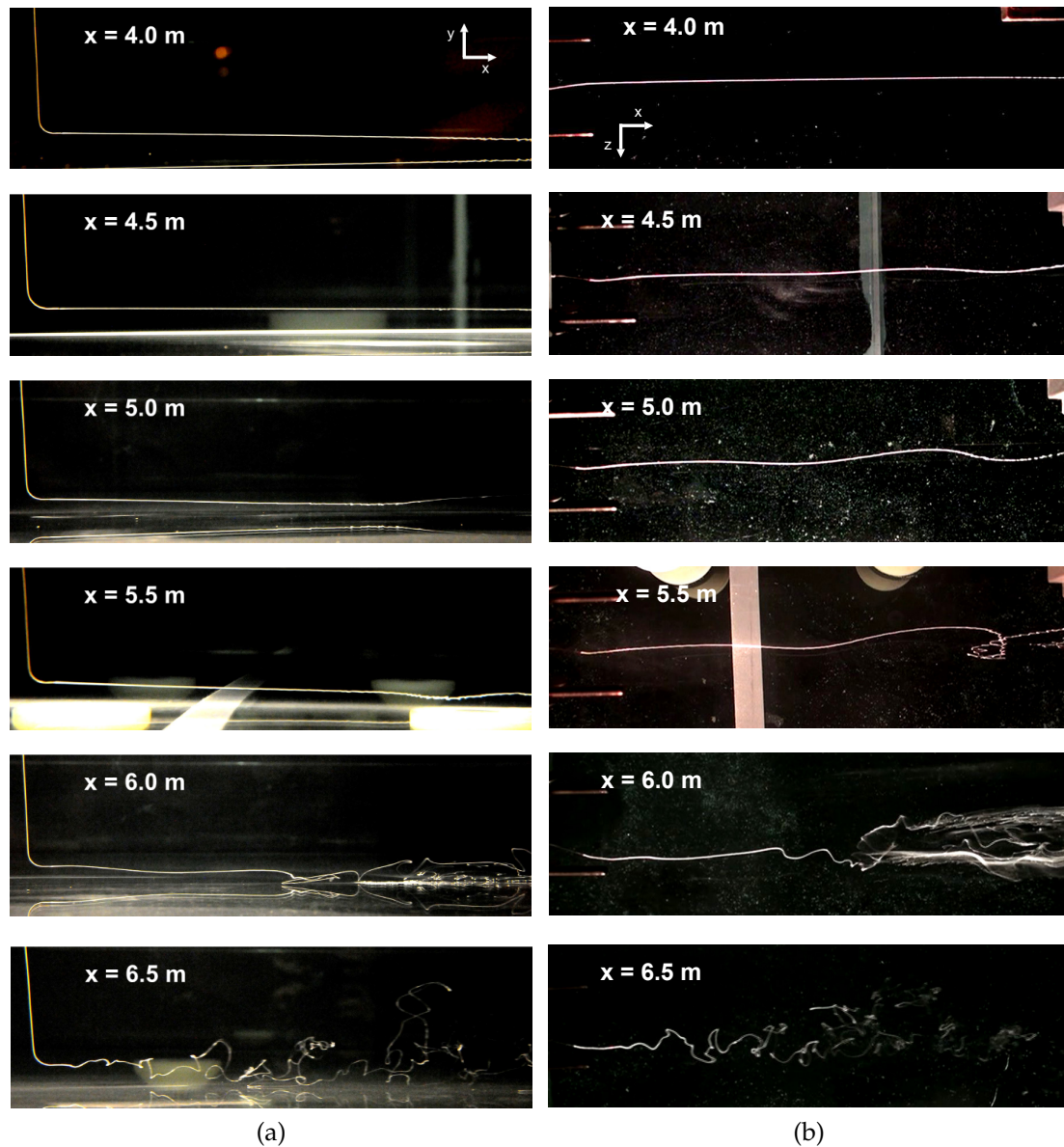
Figure B.2: Flow visualizations of laminar-turbulent transition on the flat plate by dye-streaks observed in (a) spanwise direction (b) wall-normal direction. (a) and (b) were captured independently
