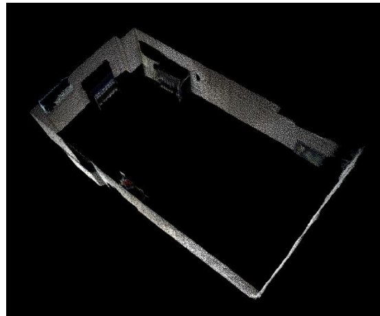
Pre-processed point cloud. Furniture is fully removed by means of a selective height filter ( 1.5\text{m} < h < 2.5\text{m} ). Remaining clutter is removed in the binarization process.
