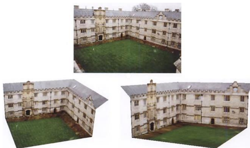
Figure 4.1 – 3D reconstruction based on a single perspective image. Top: original image (the Fellows quad, Merton College, Oxford); Bottom: 3D model from different views. (from Hartley and Zisserman (2003))
