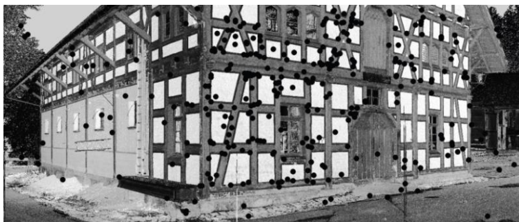
Figure 2.19 – SIFT features extracted and matched for a reflectance image. (from Böhm and Becker (2007))
