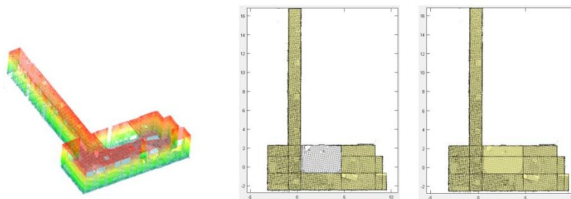
Figure 4.16 – Grammar-based reconstruction based on grammar rules derived from the point cloud. From left to right: collected point cloud, cuboid placement (top-view) with points-on-ceiling constraining and cuboid placement without points-on-ceiling constraining. (adapted from Khoshelham and Díaz-Vilariño (2014))
