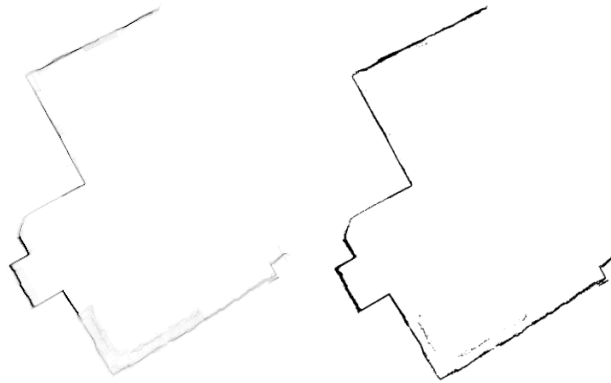
Figure 5.7 – Grayscale and binary orthographic projected image for a sample point cloud.
