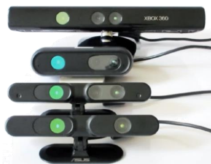
Figure 2.9 – Range cameras based on the PrimeSense technology. Top to bottom: Microsoft Kinect, PrimeSense PSDK, ASUS Xtion Pro Live and ASUS Xtion Pro. (from Böhm (2014))
