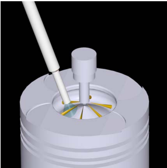
OM611: Kolbenposition in OT
