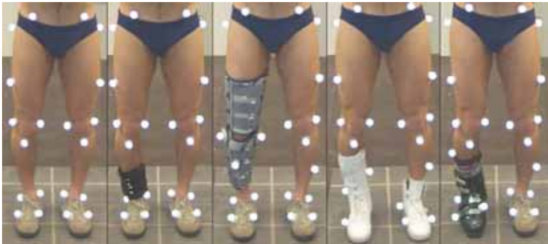
Figure 3.4: Mechanical disturbances on subject 1 from left to right: undisturbed, weight attached to the right ankle, right knee immobilization, right ankle immobilization, and ski boot on right foot.
